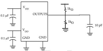
For parameter  $t_8$  (output slew rate) on -1H devices
