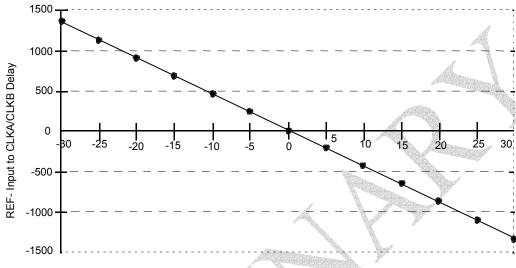
Output Load Difference: FBK Load - CLKA/CLKB Load (pF)
